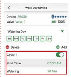
Add cycle (up to 30 watering cycles), select desired start time and watering duration.
