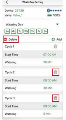
Delete cycle if needed by tapping the Delete Key, then select the trash bin of the cycle you want to remove.
