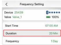
Tap "Duration" and scroll up or down to select your desired watering time. Then press the "OK" key
