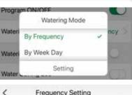
tap the "Setting" key. By selecting Frequency, you can have the device run multiple times in one day
