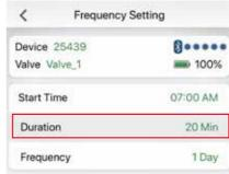
Tap "Duration" and scroll up or down to select your desired watering time. Then press the "OK" key
