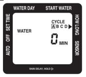
With the arrow pointing to **HOW LONG**, use the ◀ and ▶ buttons to select the length of each watering cycle. After setting HOW LONG you want to water during a selected cycle, press (CYCLE) to move to the next cycle. Repeat until **HOW LONG** has been set for each cycle.
