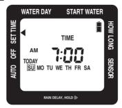
Before setting your watering schedule, you must first set the current day of the week and time. When the batteries are first installed, the arrow on the screen will point to **SET TIME**. If it is not in that position, press the button until the arrow is pointing to **SET TIME**.
