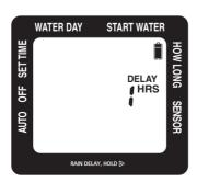
If there is rain in the forecast, you can temporarily suspend your watering program for up to 7 days using the **RAIN DELAY** feature. After the selected delay has ended, your watering program will resume automatically.
