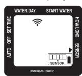
You can pair your timer with the Eden Soil Moisture Sensor (model #25417, sold separately) to monitor how wet the soil is and prevent overwatering. Set your desired moisture level and if the soil is too wet the watering schedule will be delayed.
