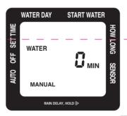
To use a hose or other watering tool, simply press the MANUAL button. Then, using the button, select the length of time you wish to water. After a few seconds, the valve will open, and then automatically close when the selected time is reached.
