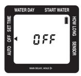
To stop watering indefinitely, press the button until the arrow on the screen points to **OFF**. The timer will not water while in this mode. The screen will display the word **OFF**.
