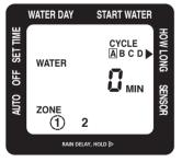
With the arrow pointing to **HOW LONG**, use the ◀ and Þ buttons to select the length of each watering cycle. After setting **HOW LONG** you want to water during a selected cycle, press (CYCLE to move ABCD)
