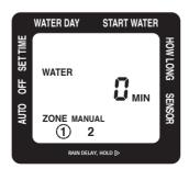
To use a hose or other watering tool, simply press the MANUAL button. Then use the ZONE out want to use.
