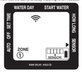
You can pair your timer with the Eden Soil Moisture Sensor (model #25417, sold separately) to monitor how wet the soil is and prevent overwatering. Set your desired moisture level and if the soil is too wet the watering schedule will be delayed. Each zone of the timer can be paired with a separate sensor.
