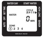
With the arrow pointing to **HOW LONG**, use the ◀ and ▶ buttons to select the length of each watering cycle. After setting **HOW LONG** you want to water during a selected cycle, press (CYCLE to move ABCD)
