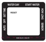
To completely erase all settings in the timer and return to the original factory settings, press the button until the arrow is pointing to **SET TIME**. Then press and hold the button for 10 seconds. The screen will display **RESET**.
