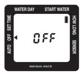
To stop watering indefinitely, press the button until the arrow on the screen points to **OFF**. The timer will not water while in this mode. The screen will display the word **OFF**.
