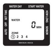
To use a hose or other watering tool, simply press the MANUAL button. Then use the ZONE button to select which zone you want to use.
