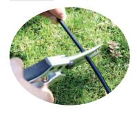
Place the drip nozzles at their desired location. Then, using a scissors, cut the tubing to the correct length to reach the nozzle.
