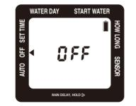
To stop watering indefinitely, press the S button until the arrow on the screen points to **OFF**. The timer will not water while in this mode. The screen will display the word **OFF**.
