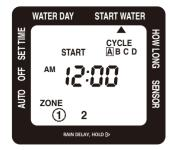
With the arrow pointing to **START WATER** on your screen, **CYCLE A** should be highlighted, use the *◄* and ▷ buttons to select the first watering time. You can select up to four independent start times **(CYCLE A, B, C, D).**
