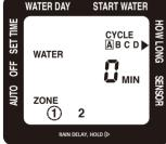
With the arrow pointing to **HOW LONG**, use the **4** and **b** buttons to select the length of each watering cycle. After setting **HOW LONG** you want to water during a selected cycle, press **CYCLE** to move to the next cycle. Repeat until **HOW LONG** has been set for each cycle.
