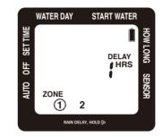
If there is rain in the forecast, you can temporarily suspend your watering program on both zones for up to 7 days using the **RAIN DELAY** feature. After the selected delay has ended, your watering program will resume automatically.
