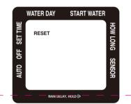
To completely erase all settings in the timer and return to the original factory settings, press the 🏂 button until the arrow is pointing to **SET TIME**. Then press and hold the 🛞 button for 10 seconds. The screen will display **RESET**.
