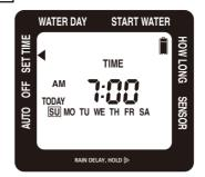
Before setting your watering schedule, you must first set the current day of the week and time. When the batteries are first installed, the arrow on the screen will point to SET TIME. If it is not in that position, press the 💪 button until the arrow is pointing to SET TIME.
