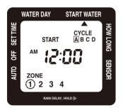
With the arrow pointing to **START WATER** on your screen, **CYCLE A** should be highlighted, use the ◀ and ▶ buttons to select the first watering time. You can select up to four independent start times (**CYCLE A. B. C. D).**
