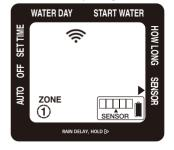
You can pair your timer with the Eden Soil Moisture Sensors (model #25417, sold separately) to monitor how wet the soil is and prevent overwatering. Set your desired moisture level and if the soil is too wet the watering schedule will be delayed.
