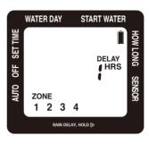
If there is rain in the forecast, you can temporarily suspend your watering program on both zones for up to 7 days using the **RAIN DELAY** feature. After the selected delay has ended, your watering program will resume automatically.
