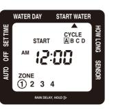
With the arrow pointing to **START WATER** on your screen **CYCLE A** should be highlighted, use the ◀ and ▶ buttons to select the first watering time. You can select up to four independent start times (CYCLE A, B, C, D).
