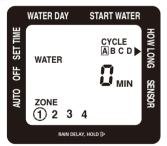
With the arrow pointing to **HOW LONG**, use the ◀ and ▶ buttons to select the length of each watering cycle. After setting **HOW LONG** you want to water during a selected cycle, press (CYCLE) to move to the next cycle. Repeat until **HOW LONG** has been set for each cycle.
