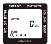
To use a hose or other watering tool, simply press the MANUAL button. Then use the ZONE button to select which zone you want to use.
