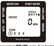
With the arrow pointing to **HOW LONG**, use the ◀ and ▶ buttons to select the length of each watering cycle. After setting **HOW LONG** you want to water during a selected cycle, press (CYCLE) to move to the next cycle. Repeat until **HOW LONG** has been set for each
