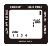
If there is rain in the forecast, you can temporarily suspend you atering program on both zones for up to 7 days using the RAIN **DELAY** feature. After the selected delay has ended, your watering
