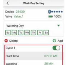
Add cycle (up to 12 watering cycles), select desired start time and watering duration.
