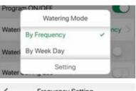
Select "By Frequency", then tap the "Setting" key. By selecting Frequency, you can have the device run multiple times in one day
